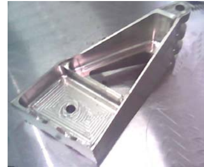
View of the Component after completion of machining
