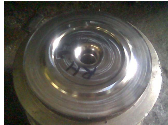
View of the Die after completion of machining
